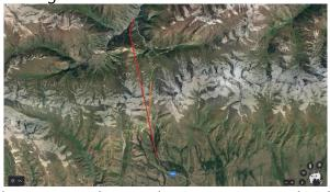
The alternative tunnel will avoid the serpentine at the entrance and exit of the existing tunnel and reduce the distance of 34 km to 11 km, reduce the time to pass the existing tunnel and serpentine from 2 hours to 11 minutes. and the spent fuel for trucks from 17 liters to 3.6 liters.
